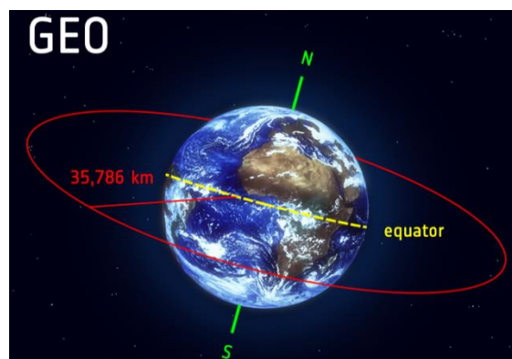
Fig 1: Geostationary Earth Orbit (GEO)
