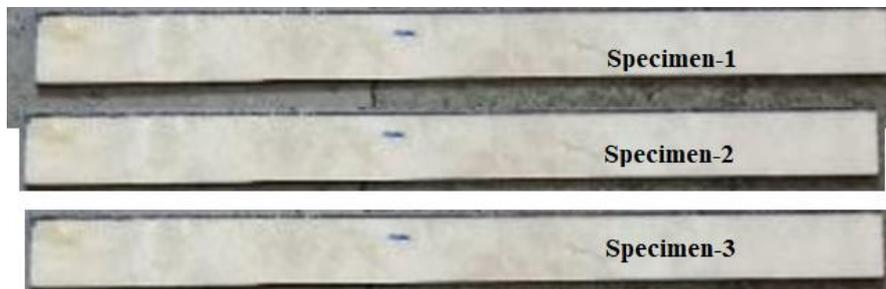
**Figure 2:** Fabricated GFRP composite test specimens
