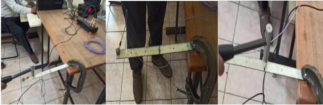
Figure-2(b): Stages of vibration testing of GFRP composites
