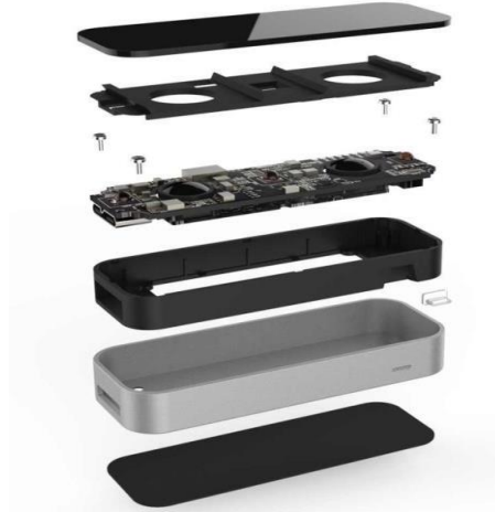
Figure 3: (Courtesy - Internet): Components of Leap Motion Controller
