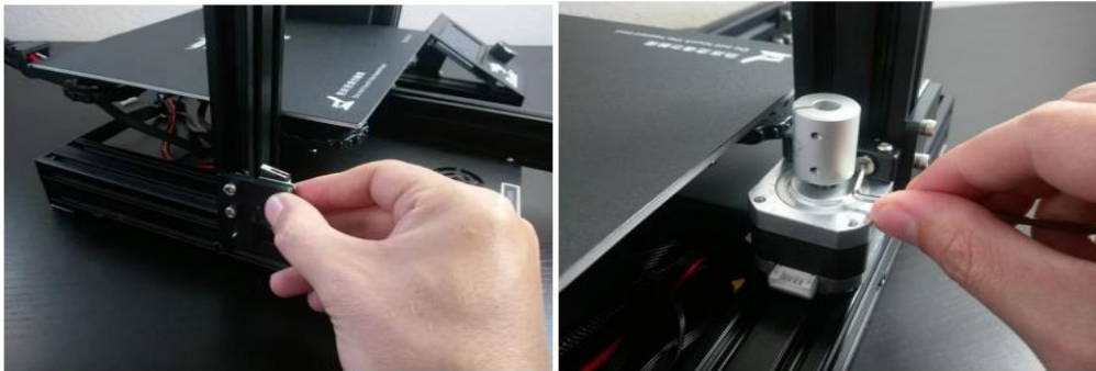
Fig 3: Z limit switch and Z motor Assembly
