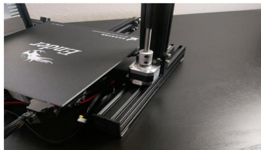
Fig 4: Inserting Lead screw.
