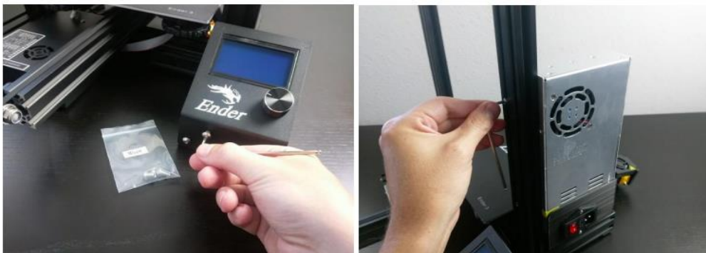
Fig 2: LCD and Power supply Assembly.
