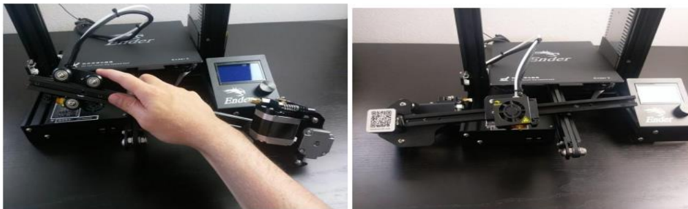
Fig 6: Positioning of gantry
