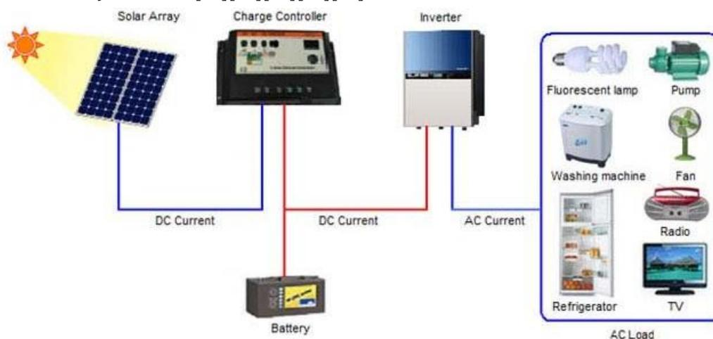
**Figure 1:** A typical solar inverter system. [36]
