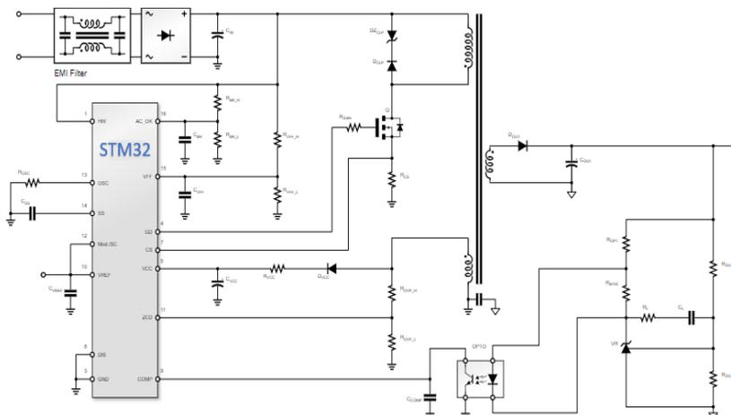
Figure 4: Solar inverter with the STM32 Microcontroller circuit diagram drawn in the eDesignSuite.
