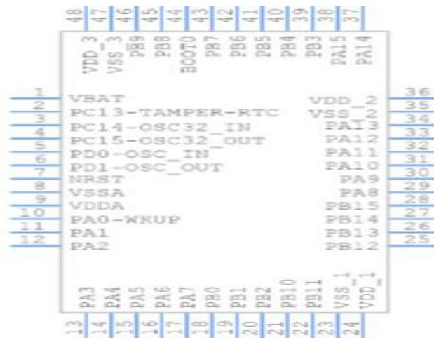
Figure 3: STM32 F100 Microcontroller circuit diagram
