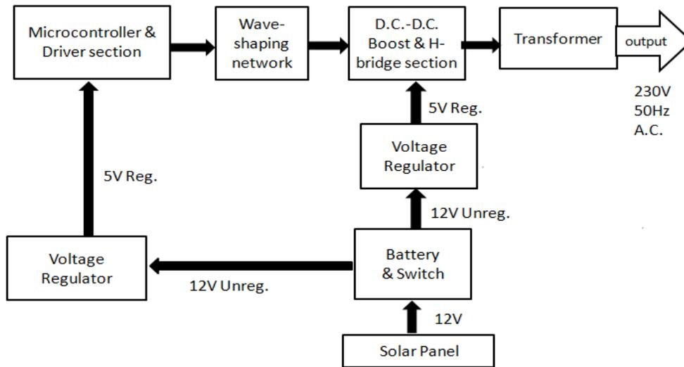
Figure 2: Block Diagram of Microcontroller based solar powered inverter [37]
