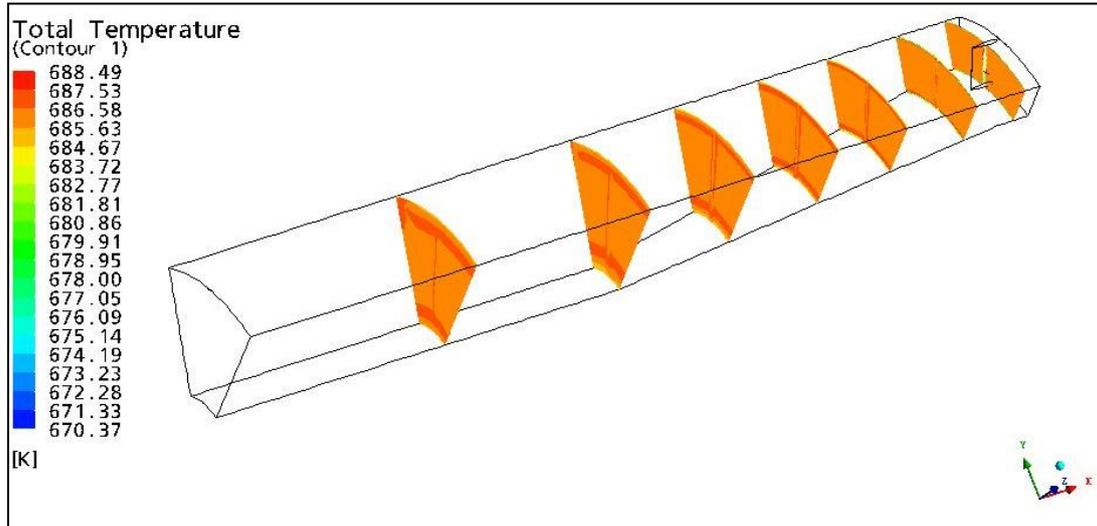
**Fig 19: Contours of Total temperature (With struts)**
