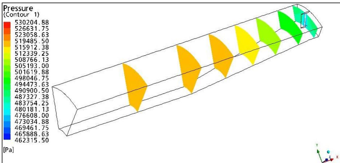
**Fig 18:** Contours of Static pressure (With struts)
