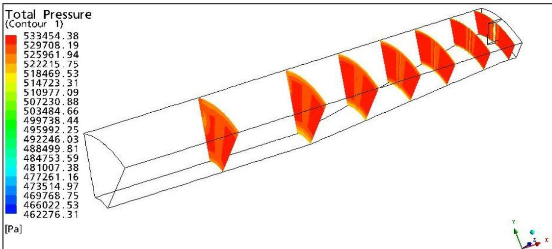
**Fig 17:** Contours of Total pressure (With struts)
