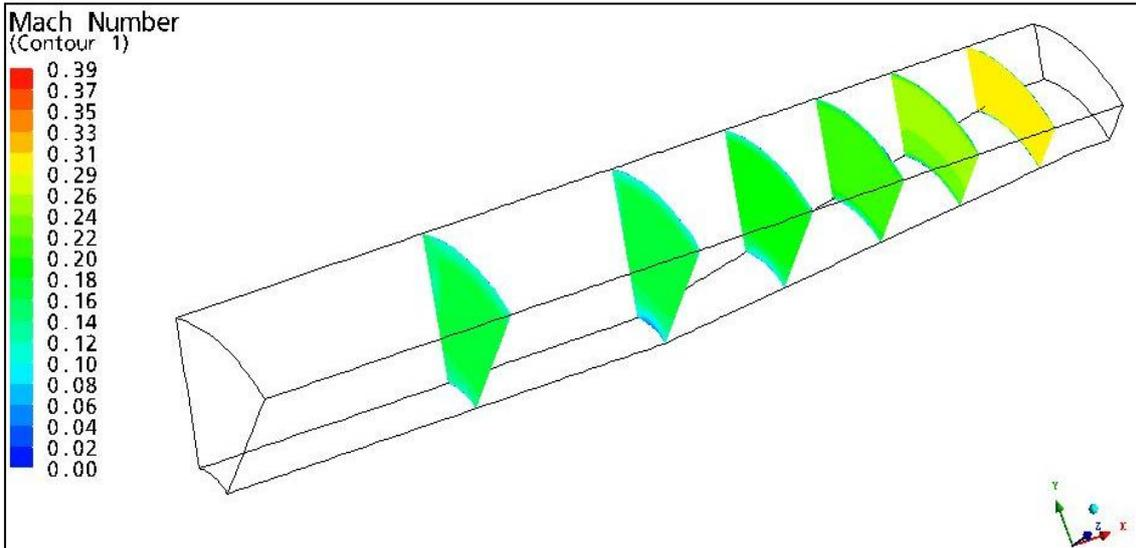
**Fig 16:** Contours of Mach number (Without struts)
