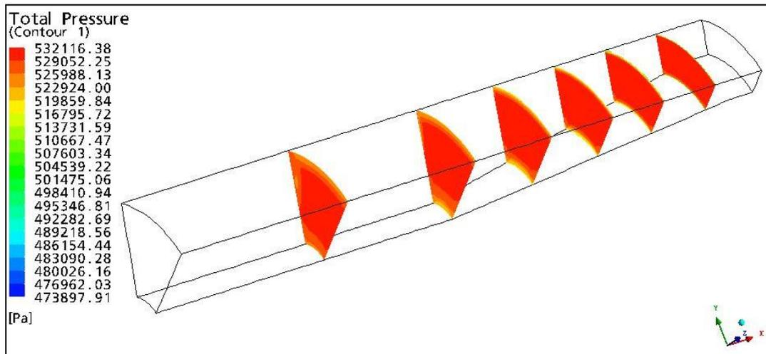
Fig 11: Contours of Total pressure (Without struts)
