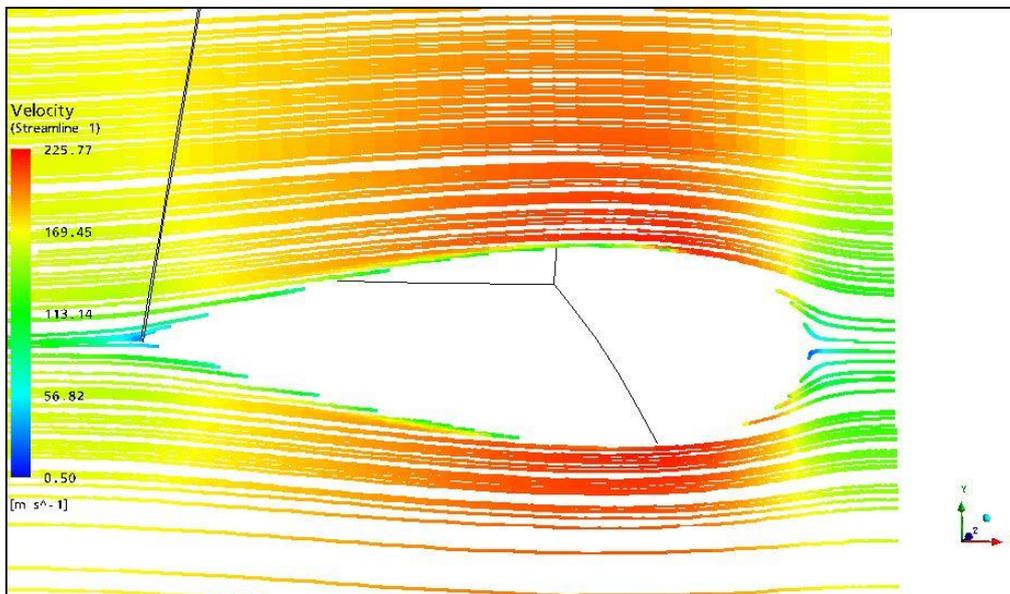
Fig 23: Stream lines around the airfoil strut
