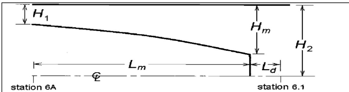
Fig 6: Geometry of the Diffuser duct (Reference, Aircraft Engine design, Jack D. Mattingly)
