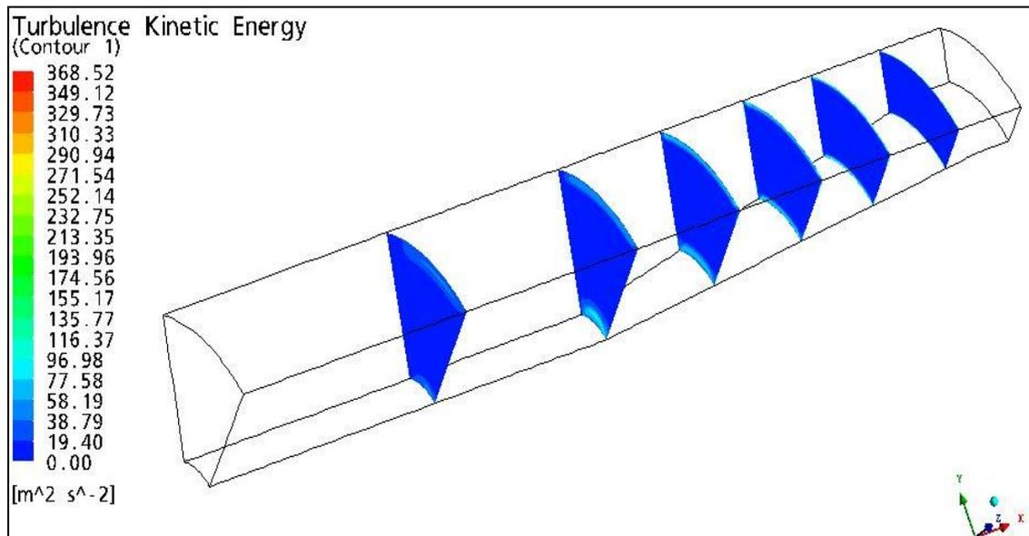
Fig 15: Contours of Turbulence Kinetic Energy (Without struts)
