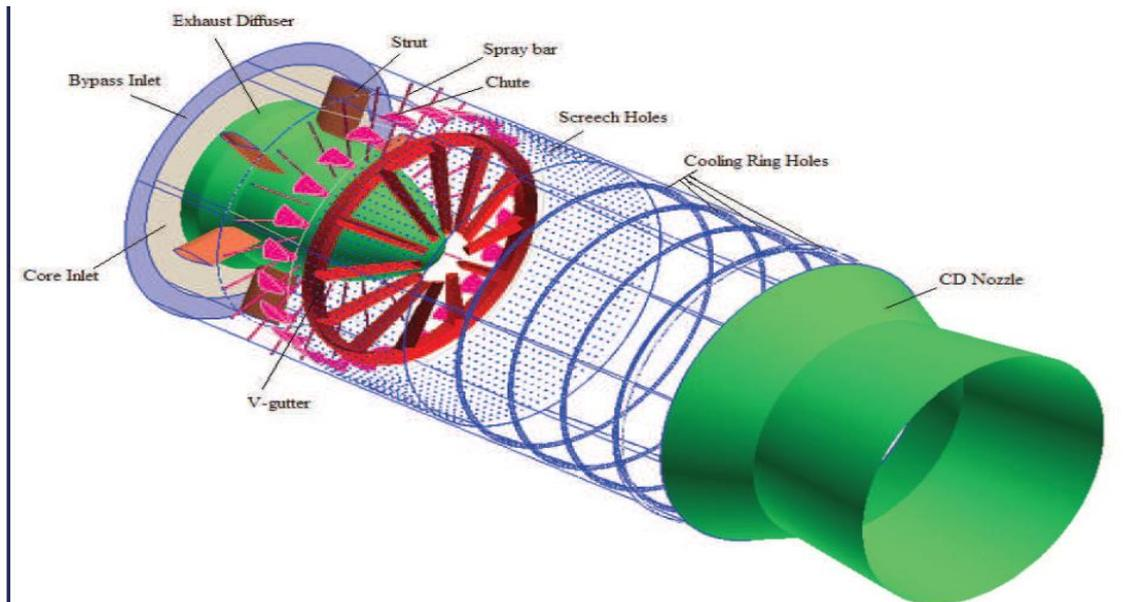
Fig 5: CAD model of the afterburner (2)
