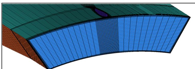
**Fig 10:** Mesh resolved near the wall region and around the airfoil to capture the viscous effects
