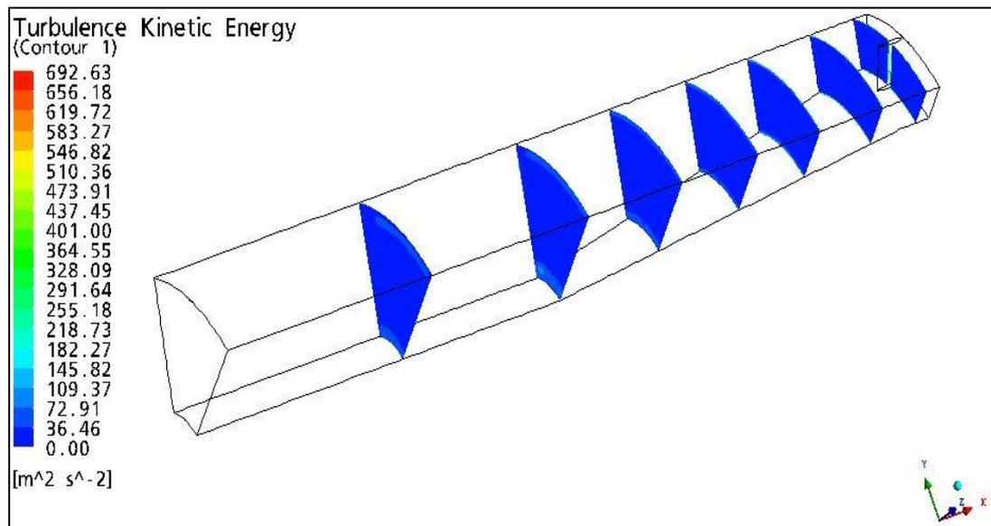
**Fig 21: Contours of Turbulence Kinetic Energy (With struts)**
