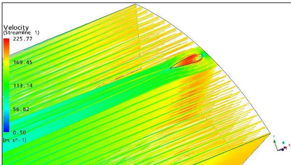
Fig 24: Stream lines around the airfoil strut (Sectional view)
