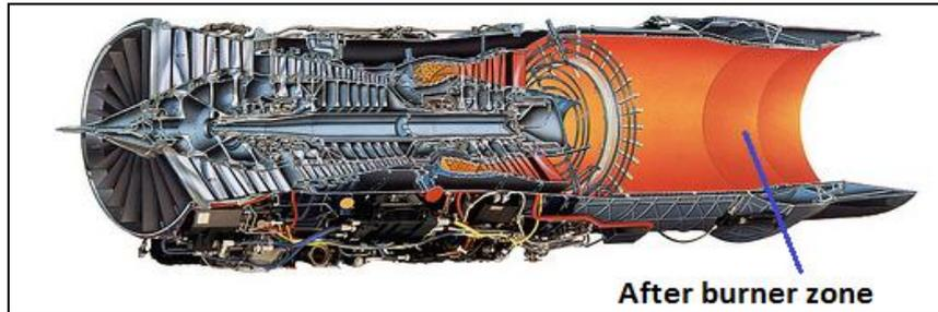
Fig 4: Sectional view off a Pratt & Whitney Turbojet Engine with after burner
