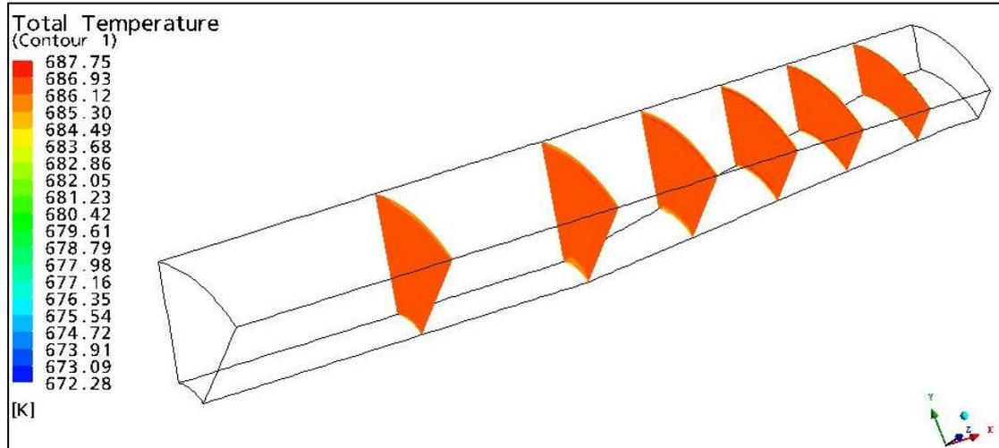
Fig 13: Contours of total temperature (Without struts)
