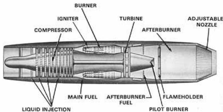
Fig 2: Gas turbine assembly with afterburner
