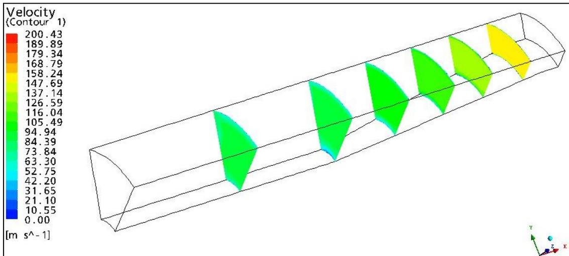
Fig 14: Contours of velocity (Without struts)
