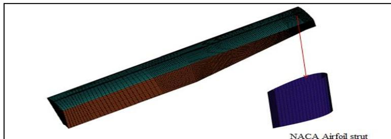
**Fig 8:** Computational domain of the after burner diffuser duct with struts(45 Degree Sector)
