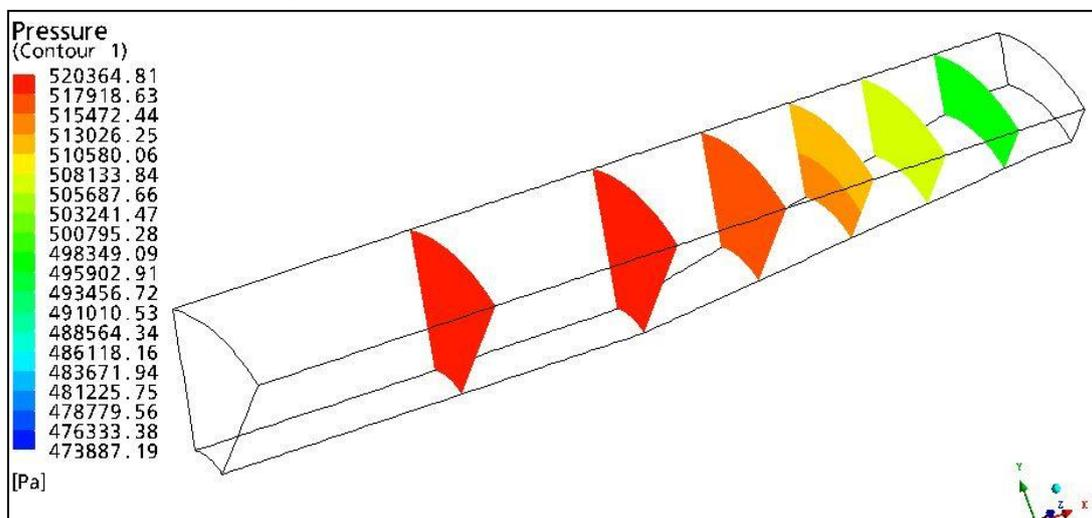
Fig 12: Contours of static pressure (Without struts)
