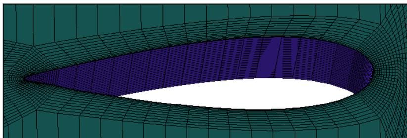
**Fig 9.** Body-fitted grid generated around the Airfoil Strut
