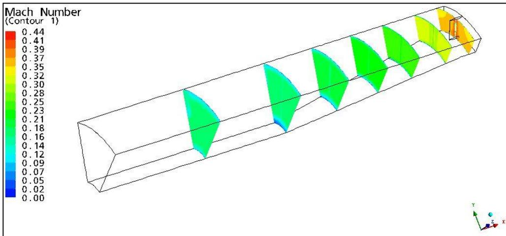
Fig 22: Contours of Mach number (With struts)
