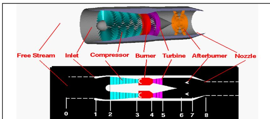
Fig 3: Schematic of a Turbojet Engine with after burner
