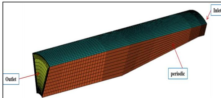
**Fig 7:** Computational domain of the after burner diffuser duct without struts(45 Degree Sector)
