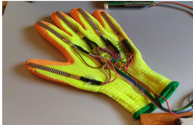
Fig 3: Glove with flex sensors
