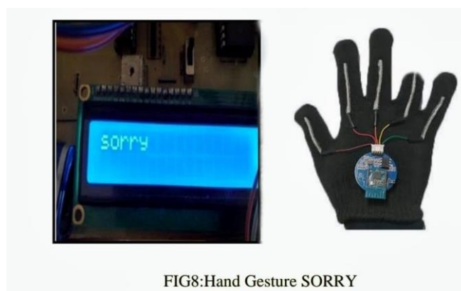
Fig 8: shows that the Ring finger is bent and Lcd shows the message Sorry
