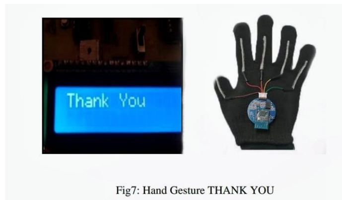
Fig 7: shows that the thumb is bend and Lcd shows the message Thank You
