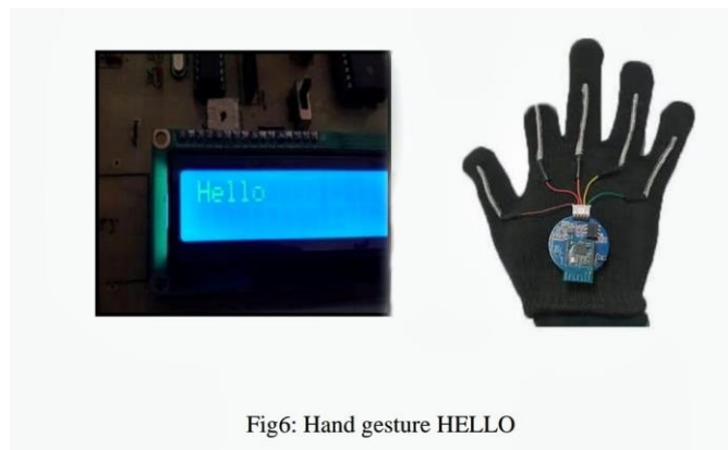
Fig 6: Shows that the Index finger is bent and Lcd shows the message Hello
