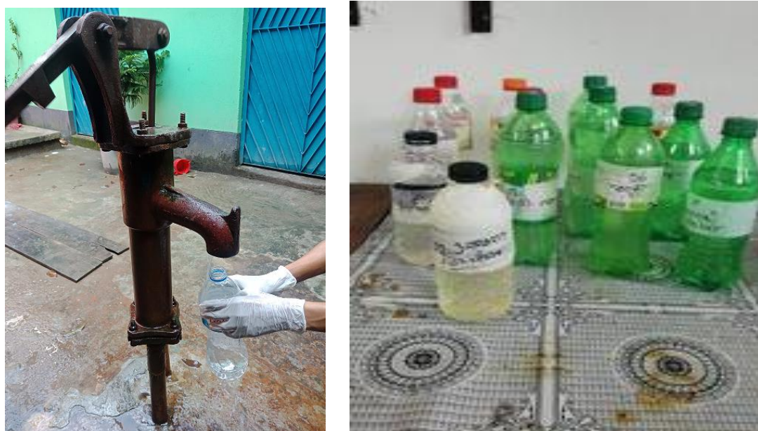
Figure 2.1: Collection and preservation of Groundwater sample
