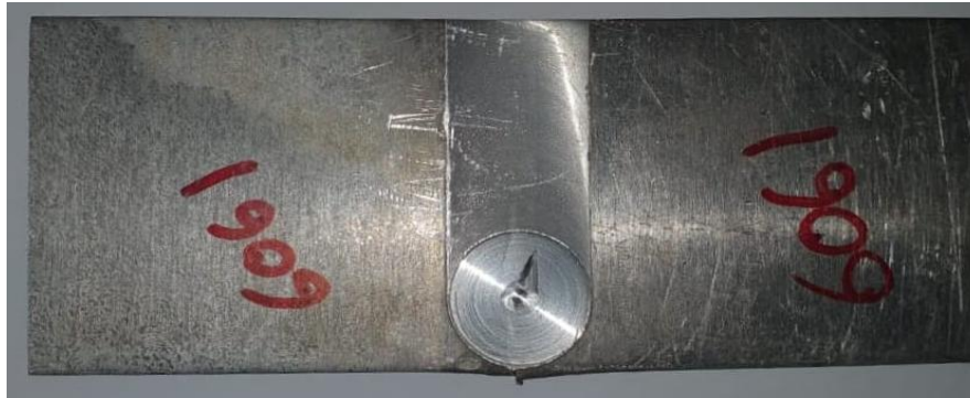
Fig 6: Compression test specimen of welded joint of aluminium alloy 6061
