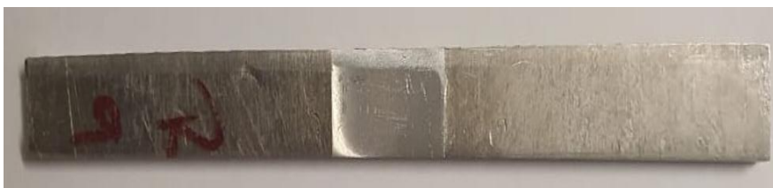
Fig 4: Brinell hardness test specimen of welded joint of aluminium alloy 6061 before test
