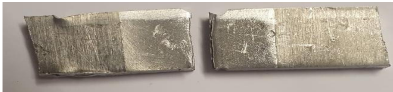
Fig 3: Impact test specimen of welded joint of aluminium alloy 6061 after test
