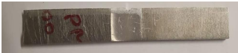
Fig 2: Impact test specimen of welded joint of aluminium alloy 6061 before test
