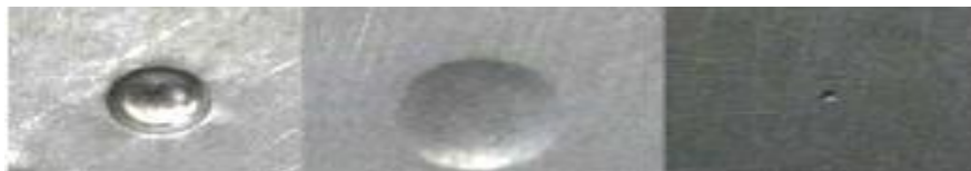
Fig 5: Brinell hardness test specimen of welded joint of aluminium alloy 6061 after test
