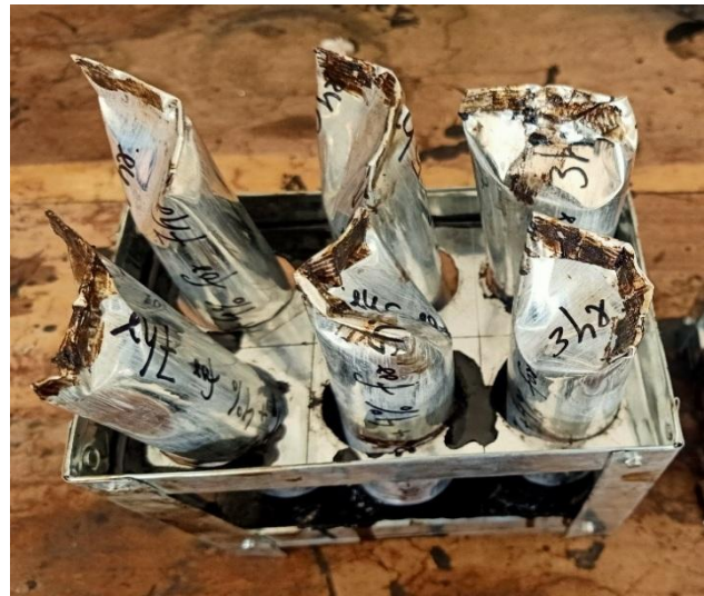
Figure 5: Aluminum Tube Containing SBS-CRMB
