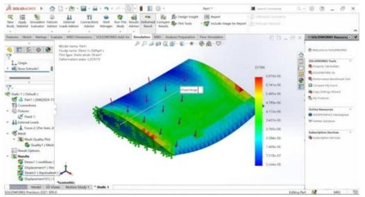
Strain analysis of turbine blade (Aluminium 2024T3) of wind turbine using Solid works (Force given is 100N and the deformation value obtained is 0.625mm)
