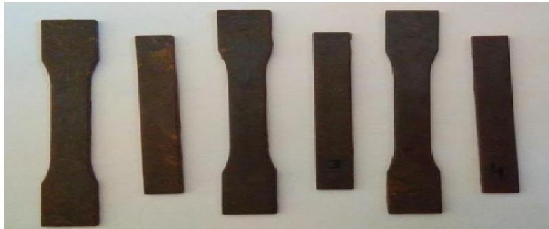
Figure 3: Samples for tensile and flexural strength testing of Sisal fiber reinforced TPU
