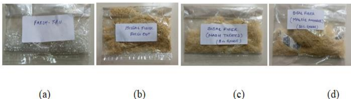
Figure 2: (a) TPU (b) Pure Sisal fiber (c) 8% wt NaOH treated sisal fiber (d) 10% wt acetone + MA treated sisal fiber
