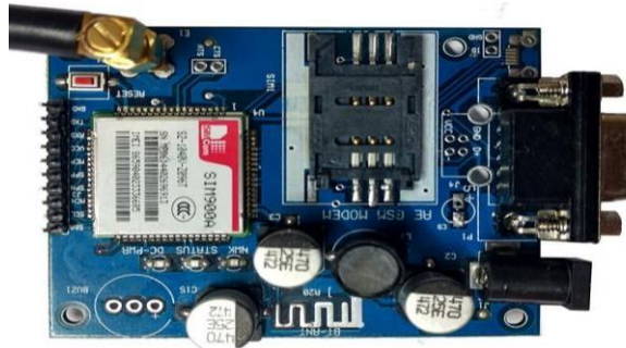
Figure 3: Overview of GSM module
