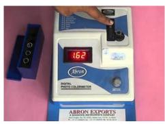
The Digital Colorimetric Method is a commonly used way to check for chlorine in drinking water.First, we take a sample of the water we want to test. Then, we add special DPD tablets or powder to the sample. These tablets contain a substance that reacts with chlorine, making the water turn pink.
