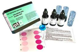
The DPD (N,N-diethyl-p-phenylenediamine) Method is a commonly used technique for detecting chlorine in drinking water.
