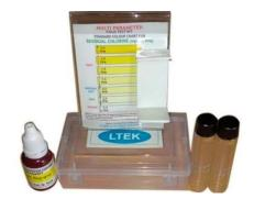
The "Chlorine Tester" uses the Acid Orthotolidine Method to determine the chlorine concentration in water. @International Research Journal of Modernization in Engineering, Technology and Science
