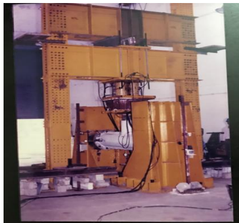
Fig. 10: Testing of repaired joint
