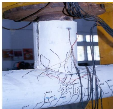
Fig. 11: Bulging out of tubular member under loading
