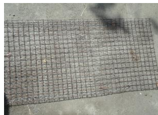
(a) Ferrocement steel reinforcement
