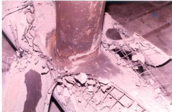
Fig. 12: Excellent bond of the HPG with the tubular member
