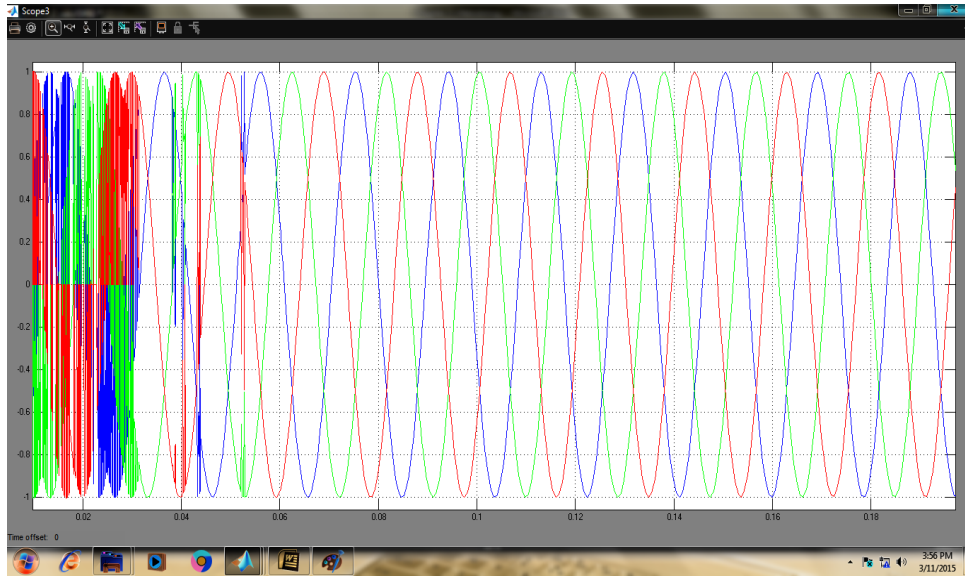
Figure 12: Rotor voltage of wind generator
