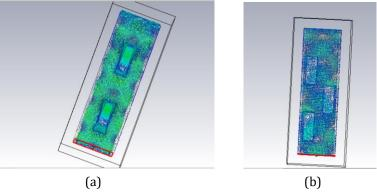
**Fig 4:-** Electric field distribution on Case-(a), Case-(b) **Table 1.** Design constraint of similar and dissimilar 2-element shunt slotted array antenna:-
