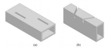
Fig. 1. Two types of radiating slots: (a) etched on the wide-wall; (b) etched on the narrow-wall.
