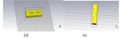
**Fig 3:-** Antenna Design. (a) two similar size lengths of slots milled on a WR90 at a similar distance from centre and aligned in a line. (b) two similar size lengths of slots milled on aWR90 at a similar distance from centre but are in zig-zag direction from each other.
