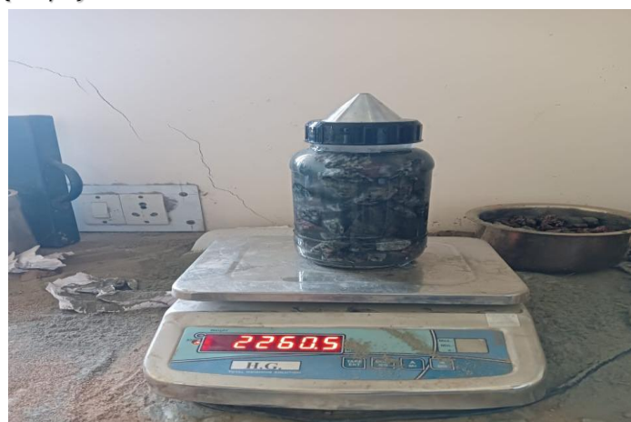
FIG 3. Weight of vessel + coarse aggregate + water ( for specific gravity and water absorption test)
