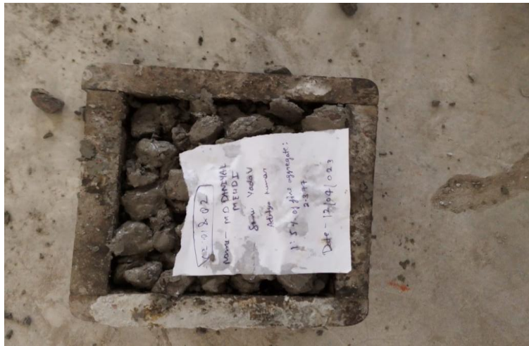
FIG 4. Casting of pervious concrete
