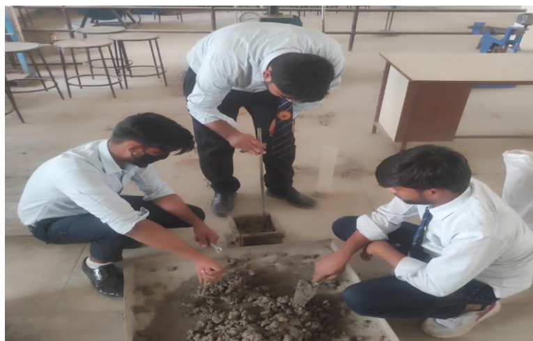
FIG 1. Mixing And Casting Of Pervious Concrete
