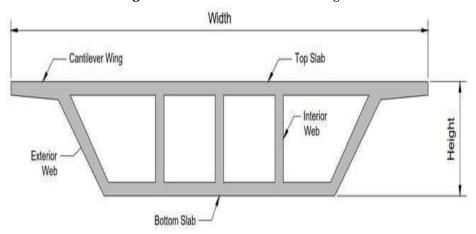
Figure 2: Cross Section of Highway Bridges.
