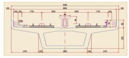
Figure 1: Cross Section Of Metro Bridges.
