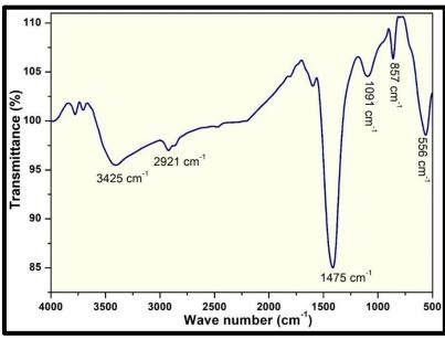
**Figure 3.4:** FT-IR spectra of CdFe<sub>2</sub>O<sub>4</sub> nanoparticle synthesized by the impact of bio-fuel in combustion process.
