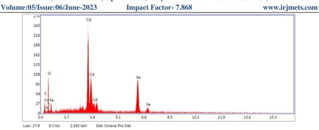
Figure 3.3: EDAX of CdFe<sub>2</sub>O<sub>4</sub> (Cadmium Ferrite) nanoparticles
