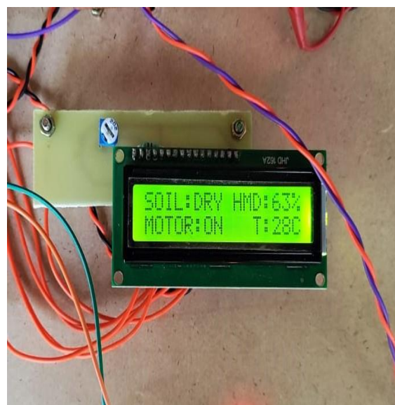
Figure 3: When moisture is LOW
