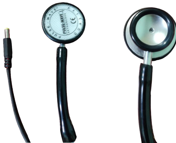
Figure 2 – Stethoscope head with microphone
