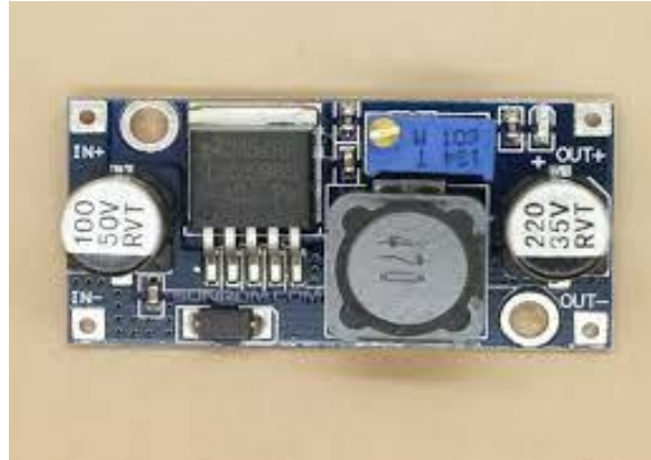
LM2596 DC-DC Buck Converter
