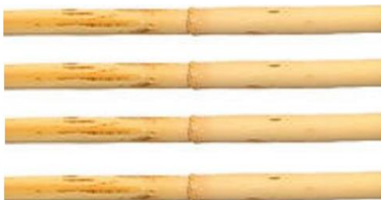
Figure 22: Bamboo boom used for Quadrotor
