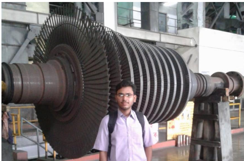
Figure 1: Industrial Steam Turbine
