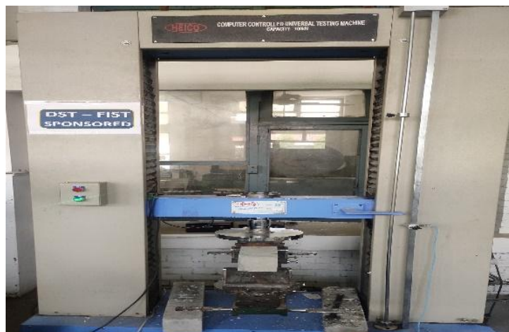
Fig.-1: Flexural Test on UTM
