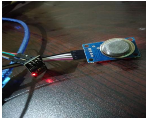
Fig-4.1: MQ 135 and ESP 8266 sensors
