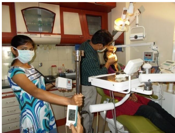
Figure-2: Air Sampling conducted (Hi-Air sampler) during patient’s procedure in dental clinic and also recorded the maximum, minimum temperature and relative humidity by using hygrometer.
