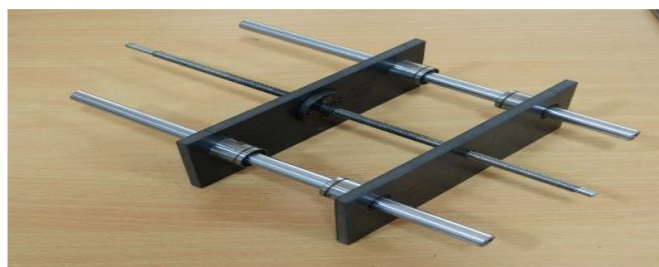
Figure 4 Assembly of linear bearing & guide rods
