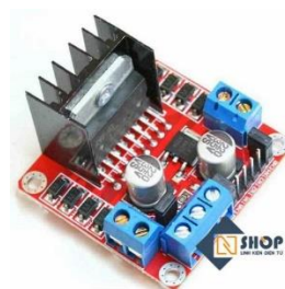
Figure 5: L298N DC motor driver circuit
