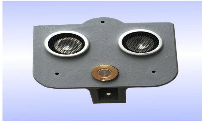
Figure 7: Ultrasonic Sensor and Nozzle Assembly
