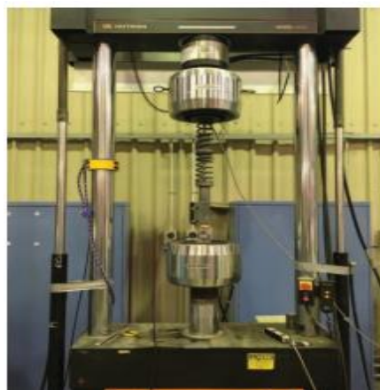
Figure 7: The testing system with the proposed MRF damper [6]
