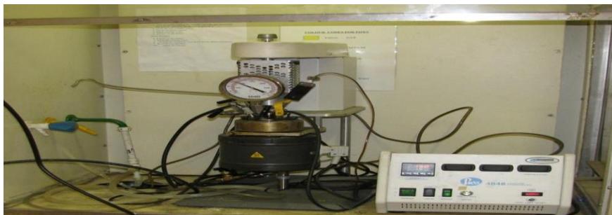
Figure 3.1: Parr reactor for the laboratory preparation of biodiesel
